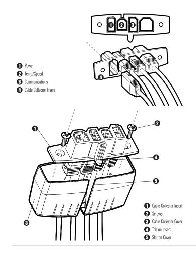
Plug Cable Connector Assembly to Back of Control Head
